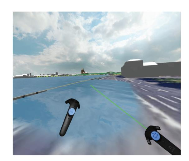
VR rendering of physically correct flooding levels, using a validated, robust simulation [2].
